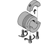
9. Push couplings as far as possible onto the drive shafts.
