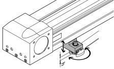
10. Tighten screws. Apply counter pressure to the adjusting bolt.
