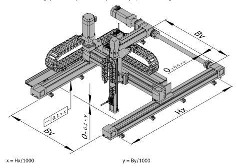
2. Lightly clamp X-axis with energy chain to the mounting surface.
