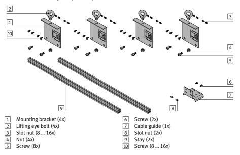
• Fasten lifting eye bolts to mounting brackets with the nut.
