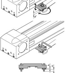
11. Make sure there is sufficient screw-in depth m of the screw (→ Table).
