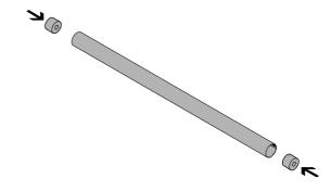
2. Place connecting tube into the couplings.
