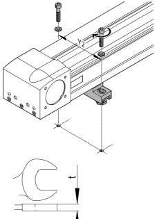
7. Use spanner with t < 5 mm. If t > 5 mm, the maximum height compensator is smaller by the difference (t - 5) mm.
