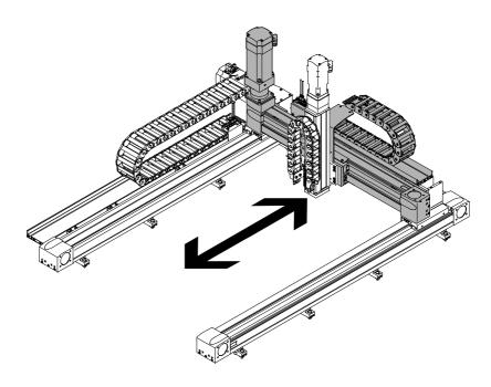
13. Move Y-module into the middle of the X-axes.
