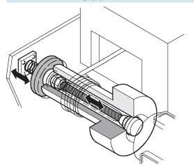
The friction-free muscle allows uniform and gentle braking of the pay-out reel, ensuring highly precise winding at constant speed. Control is provided by a proportional control valve whose signals are regulated via force sensors.
