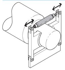
The fluidic muscle is setting new standards in applications that require fast response times. The emergency stop for rollers demands both speed and force. Long machine downtimes in the event of malfunctions can thus be prevented.
