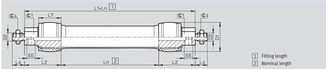
AM-RM – pneumatic connection, axial and radial
