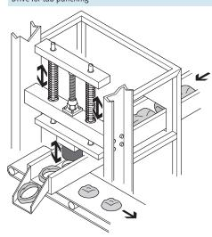
Very high cycle rates are possible with the muscle, on the one hand because of its low weight and on the other because it has no moving parts (e.g. piston). The simple construction – one muscle pretensioned using two springs – replaces a complicated toggle lever clamping system using cylinders. This makes a frequency increase of 3 to 5 Hz possible. Over 50 million load fluctuations can be achieved in this way.
