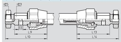
EA/BA-EG/BG - pneumatic connection, radial with threaded rod, one end/both ends
