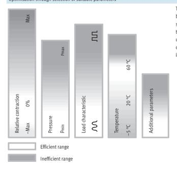
The service life of the fluidic muscle is between 100000 and 10 million switching cycles for typical applications. Optimisations can be made using the information from the left diagram. The service life thus increases due to a reduction in the relative contraction (use of a longer muscle). It is also recommended that the pressure be reduced, which is possible because the fluidic muscle is more powerful with lower relative contraction. This measure also improves the service life.
