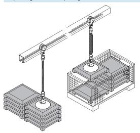
Approximate intermediate positions? No problem with pressure regulation. The workpieces can be raised or lowered as required by pressurising or exhausting the muscle via a hand lever valve. Muscle lengths up to 9 m facilitate various types of application.
