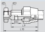
ER/BR-EG/BG - pneumatic connection, radial with threaded rod, one end/both ends
