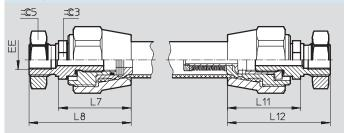
ER/BR - pneumatic connection, radial, one end/both ends
