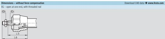
EA/BA – pneumatic connection, axial, one end/both ends
