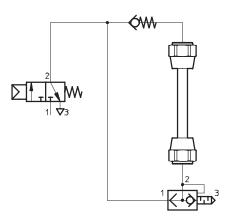
The service life of the Fluidic Muscle depends on the contraction, the operating pressure and the temperature. High operating frequencies or high loads can lead to a temperature rise. Targeted pressurisation on one side and venting on the other side enables. the thermal load on the component to be reduced and the service life of the fluidic muscle to be increased (only with fluidic muscle open at both ends).
