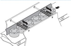
With small batch sizes, it is often necessary to adapt entire system sections to different component dimensions after a short period of time. This task can be performed with the fluidic muscle in cases where an approximate adjustment is sufficient.
