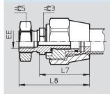
ER/BR - pneumatic connection, radial, one end/both ends
