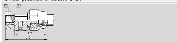
${\tt MAS-...-ER/BR-EG/BG-pneumatic\ connection,\ radial,\ with\ threaded\ rod,\ one\ end/both\ ends}$
