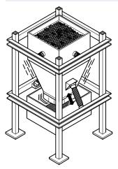
Hoppers and silos are often susceptible to problems, such as a "jamming arch" forming during feeding. In practice, discharge aids such as vibrators or knockers are used to prevent such a jam from forming. This function can be implemented with the help of the Fluidic Muscle. The frequency can be set in an infinitely adjustable manner up to 150 Hz, independently of the amplitude. This guarantees a continuous conveying process.
