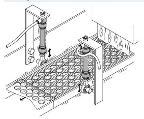
When a viscous coating agent is applied to a fixed substance carrier, a vibrating support is required to ensure even distribution over the surface. In the case of strokes of less than 1 mm, the Fluidic Muscle can achieve cycle rates of up to 150 Hz.
