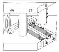
In joining processes such as those that take place in welding machines, the components to be welded are held in place by the Fluidic Muscle during the joining procedure. Here, too, the muscle can make the most of its high force combined with a small diameter.
