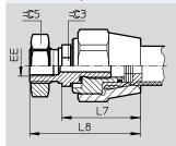
MAS-...-ER/BR – pneumatic connection, radial, one end/both ends
