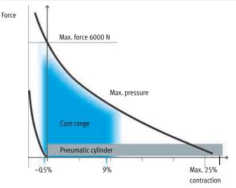
The muscle expands lengthways when it is pretensioned by an external force. When pressurised, on the other hand, the muscle contracts, i.e. its length decreases.
