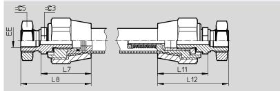
MAS-...-ER/BR – pneumatic connection, radial, one end/both ends
