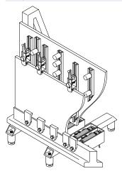
The Fluidic Muscle enables large and unwieldy workpieces, such as plates, walls and side covers, to be easily clamped so they can be machined (turning, drilling, milling). This brings out the muscle's outstanding characteristics, such as high force combined with a small diameter, frictionless and thus jerk-free movement, insensitivity to dirt (swarf, abraded particles) and hermetically sealed design.
