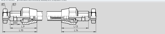
$MAS-...-EA/BA-EG/BG-pneumatic connection, \ radial, \ with \ threaded \ rod, \ one \ end/both \ ends$
