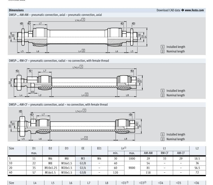
1) Tolerance < 100 mm ±1 mm, 100 ... 400 mm ±1%, > 400 mm ±4 mm.
