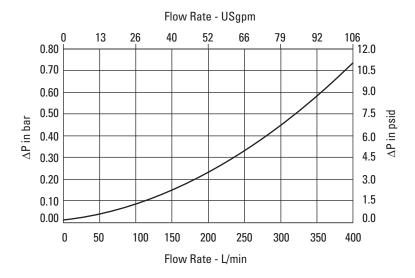
Sample  $\Delta P$  Calculation : DLR1160BE6ANBC03 - Filter assembly having '160' size filter element with micron rating code '03' at 100 L/min flow rate using a hydraulic fluid at 46 cSt viscosity & specific gravity
