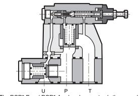
The RQR\*-P and RQR\*-A valves have not only the normal function of relief valves or safety valves but also the characteristic of freely discharging the pump flow when the set pressure value is reached.
