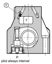
Y: plug M6x8 for external drain
