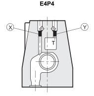
**X**: plug M5x6 for external pilot **Y**: plug M5x6 for external drain
