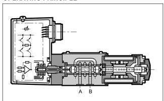
— The DXJ3 valve is a four-way servo-proportional valve where the spool moves inside a sleeve. This valve has a direct drive with a linear force motor resulting in high dynamic performances which are independent of system pressure. The spool position is controlled by a linear
