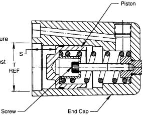
When reassembling spring centering end cap, maintain "S" dimension.
