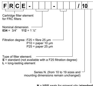
N = NBR seals for mineral oils (standard)
