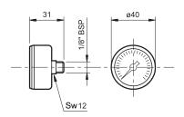
This indicator is a pressure gauge sensitive to the filter input pressure.
